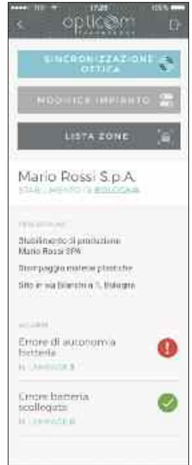
System details: Description of the system and of any lamp errors. The lamps can also be interrogated using the "optical synchronisation" push-button
